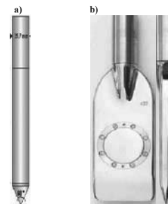
Figure 1. View of CPTu tip (a) and DMT blade (b) actually used in geotechnical investigation
