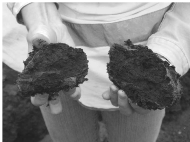
Figure 5. Pieces of peat found in jet grout spoil.
