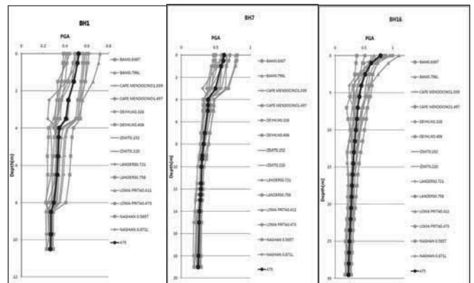
Figure 5. PGA curves for boreholes of group1.
