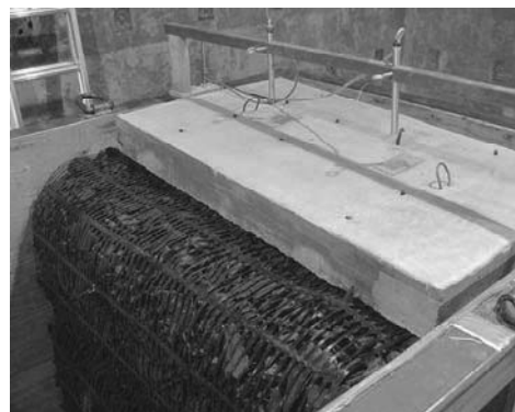
Figure 3. Constructed model MSE wall
