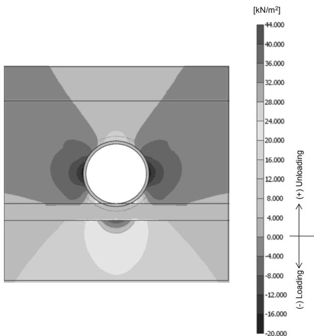
Figure 3. Stage 1, excess of pore pressure
