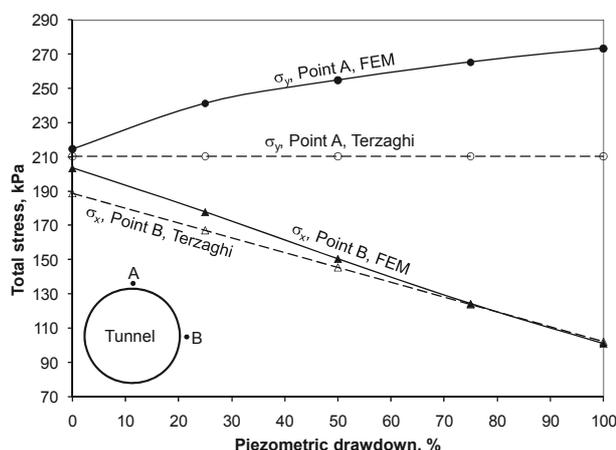
Figure 7. Variation of total stresses with piezometric drawdown
