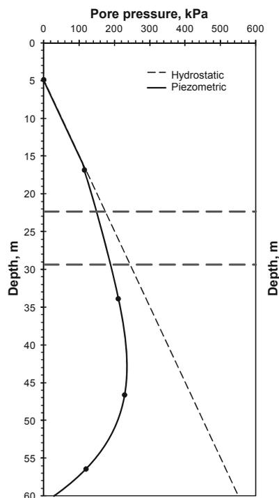
Figure 1. Pore pressure profile
