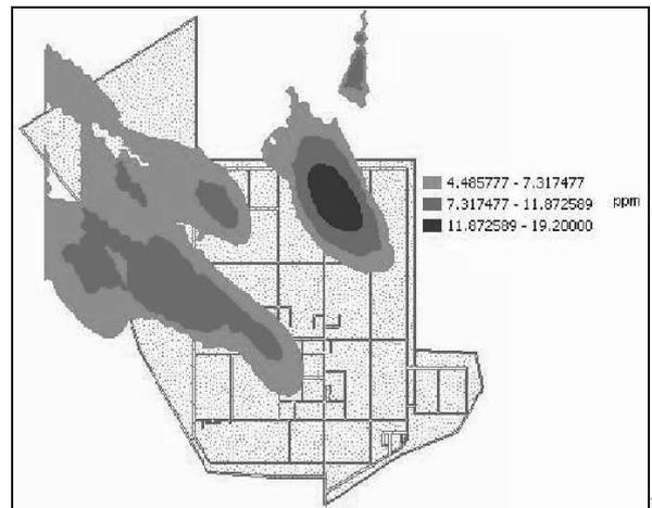
Figure 7. Hot spots of oil contamination beneath the refinery (concentrations are in terms of Total Organic Carbon).
