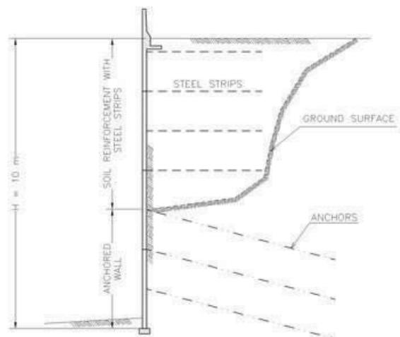
Figure 1. Typical cross-section of mixed reinforced fill-anchored wall.
