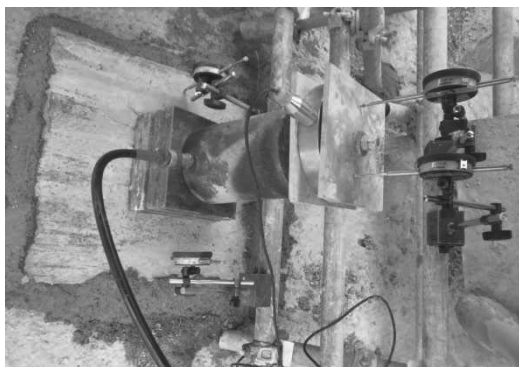
Figure 2. Typical set-up for pull-out tests.
