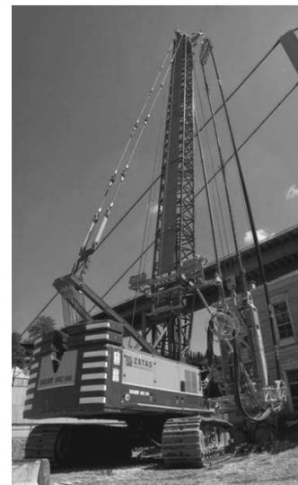
Figure 8. Diaphragm Wall Machine, Hydrofraise-Cutter
