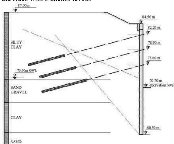
Figure 3. Cross section through the diaphragm wall
