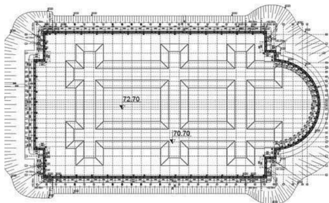
Figure 2. General layout of the diaphragm wall enclosure
