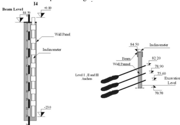
Figure 10. Inclinometer location inside the diaphragm wall
