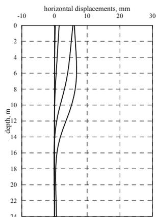
Figure 5. Horizontal displacements of the diaphragm wall
