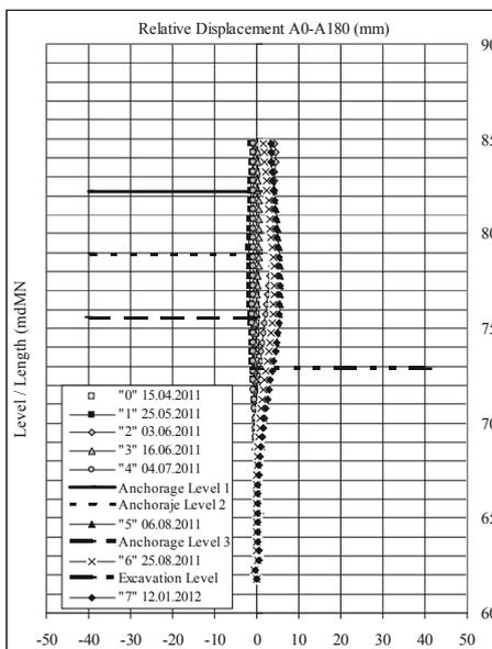
Figure 11. Inclinometer measurements for the diaphragm wall
