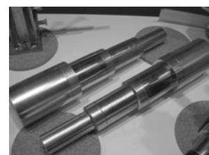
Figure 2. The steel sockets.
