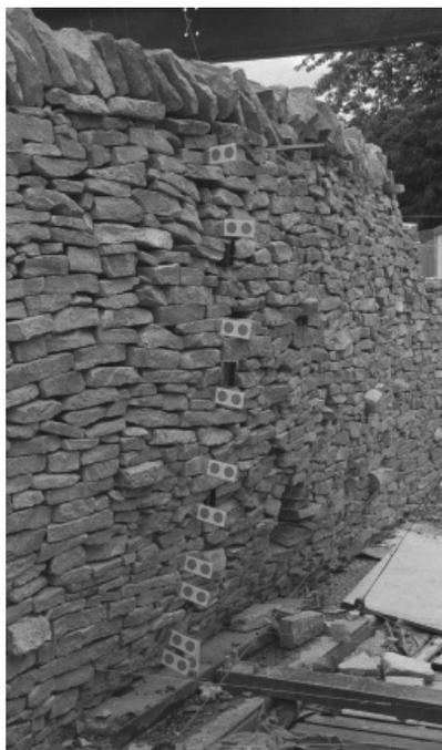
Figure 2. 2.4m high test wall at the University of Bath showing a classic bulged profile in a limestone wall of horizontal construction.
