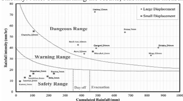
Fig. 8 Threshold value curves correlate with displacement
