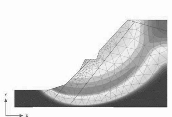
Figure 7. Total displacement
