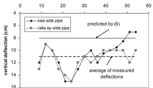
Figure 4. Comparison between measured and predicted short-term deflections
