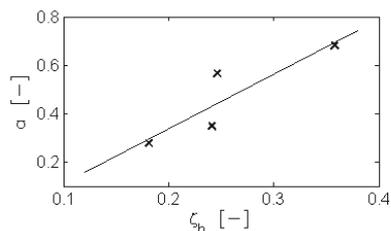
Figure 6. Fitted empirical constant  $a$  as a function of the loading magnitude  $\zeta_b$  in the four cyclic tests.
