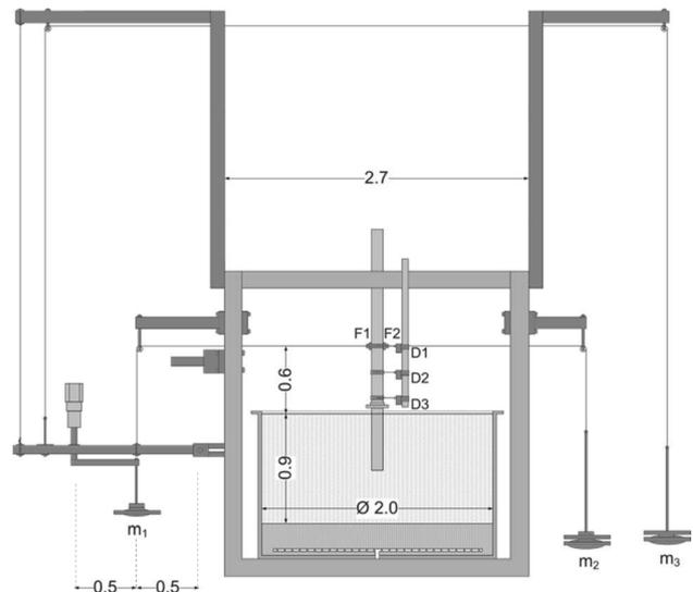
Figure 1. Sketch of the test setup. F1 and F2 refer to the two load cells, D1, D2, and D3 refer to the three displacement transducers and  $m_1$ ,  $m_2$ , and  $m_3$ , refer to the weights applied on the load hangers. All measurements are in meters.
