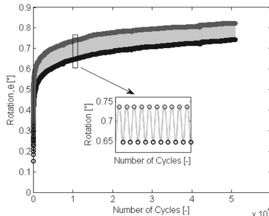
Figure 4. Rotation of the pile at soil surface as a function of the number of cycles in the test with  $\zeta_b = 0.25$ . Maximum and minimum values of the rotation are indicated by dark grey and black colouring.
