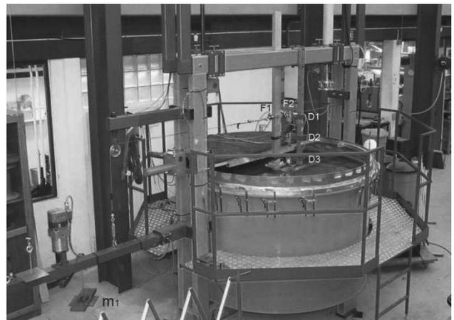
Figure 2. Test setup for cyclically long-term loaded monopiles.
