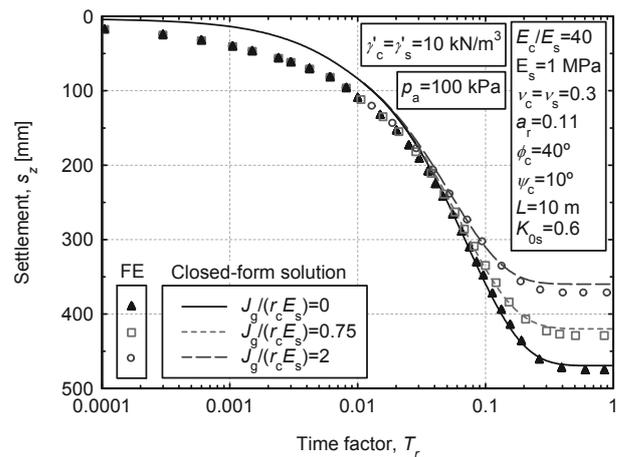
Figure 6. Time-settlement curve.
