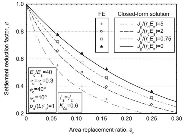
Figure 5. Settlement reduction. Influence of the encasement stiffness for different area replacement ratios.
