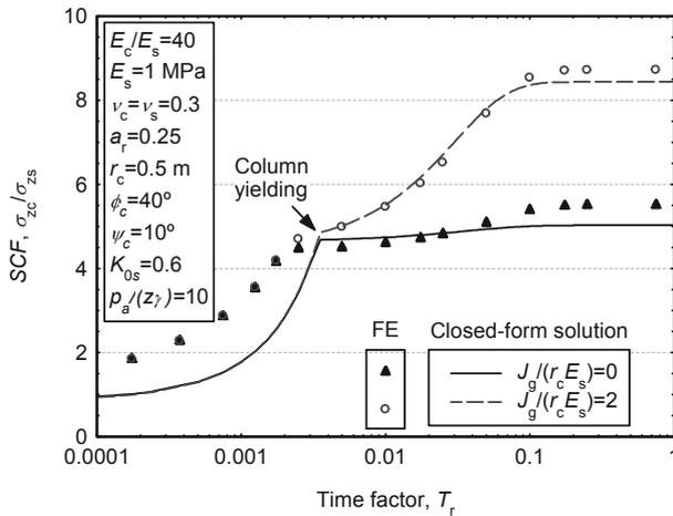
Figure 3. Stress concentration on the column with time.
