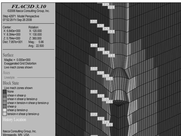
Figure 3. Plasticity zones during multi-stage filling of the stone column with crushed geomaterial at depth of 16 to 15m simulated by an equivalent static radial pressure (sub-stage IIIa, 8<sup>th</sup> ascending step of construction of the examined stone column)
