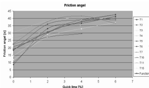
Figure 5. Increase of the friction angle at an age of 28 days, plotted against the quantity of lime
