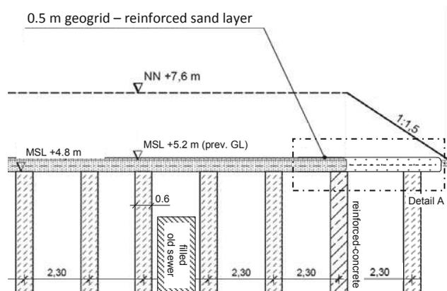
Figure 2: Cross section – piled sand layer
