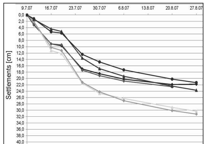
Figure 4: Development of settlement during loading phase
