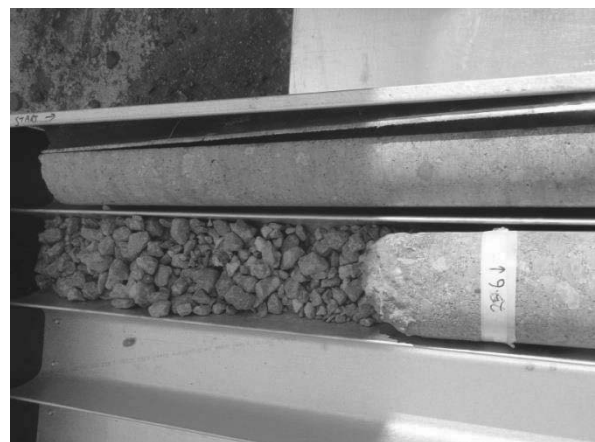
Figure 7 - Core of East Abutment NW pile
