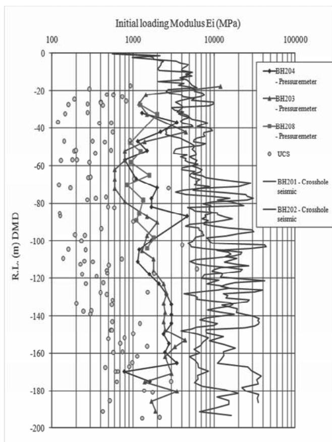
Figure 2 comparison of modulus values from UCS tests, pressuremeter and cross-hole seismic tests
