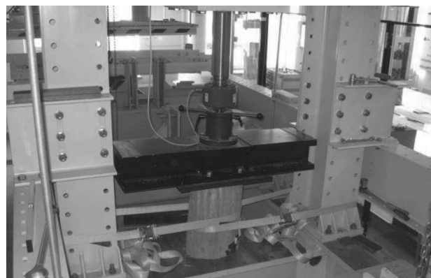
Picture 2. Test arrangement for Stress-strain behavior.
