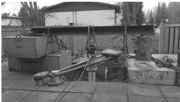
Picture 4. Arrangement of the load test in Salo 2012.
