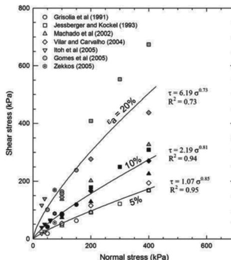
Figure 2. Summary of triaxial lab tests (Stark et al., 2009)
