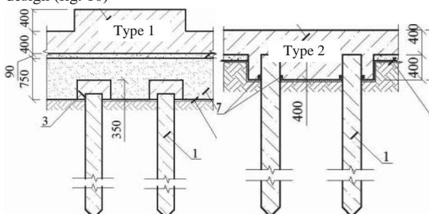
Figure 10. Foundation types for plot 17.
