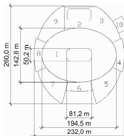
Fig. 5. Layout of Rafts of Big Ice Arena. 1. Raft of Main Arena; 2. Raft of workout arena; 3... 9 Rafts of service premises and bypass road; 10. Raft of refrigeration center.
