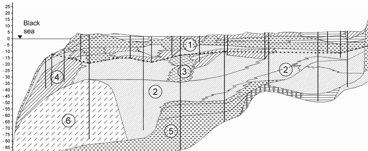
Figure. 2. Typical soil profile for Imeretin lowland.
