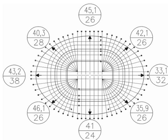
Figure 6. Mean value (mm) of measured (numerator) and analytical (denominator) settlements of arena raft footing.
