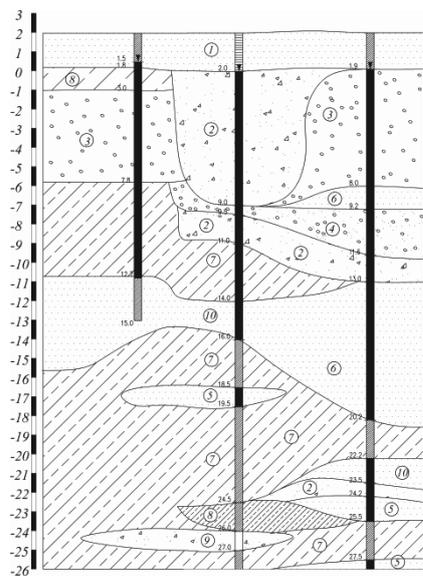
Fig. 4. Arena geological profile: 1. Coarse grained sand; 2. Gravelly soil; 3. Pebble soil with sand fill; 4. Gravelly sand 5. Fine to medium sand, with thin seams of sandy clay; 6. Sand; 7. Plastic sandy loam; 8. Sandy loam with pebbles; 9. Gravel and pebble mixture; 10. Fine sand.
