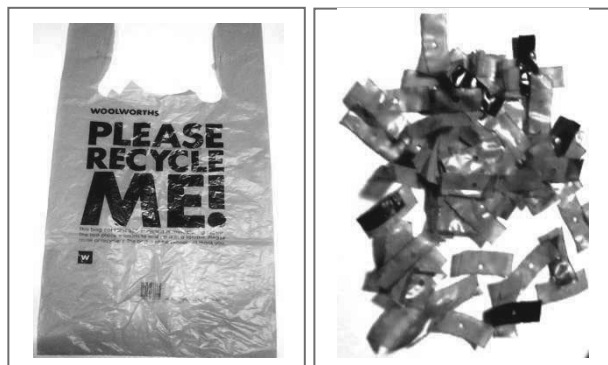
Figure 1: a) Plastic Bag b) Shredded and perforated strips
