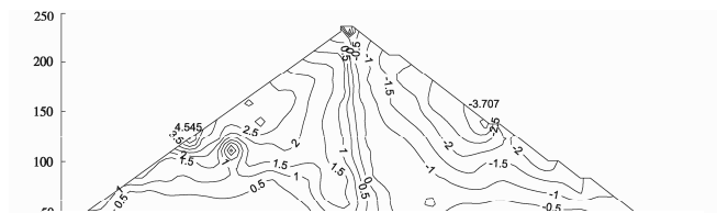
(a)Settlement difference of Bakun Dam body designed by deformation coordination method (unit: 10^{-2} )
