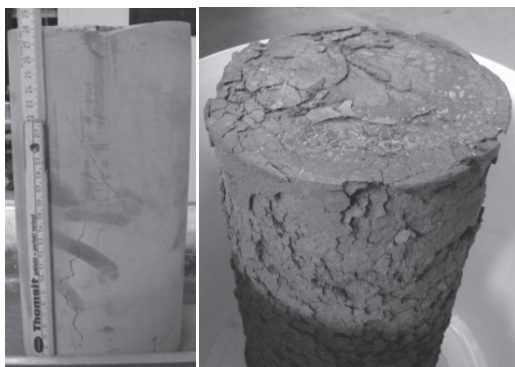
Figure 7: Alteration of a blank sample of grout material in contact with air (left) or with water (right) after two cycles
