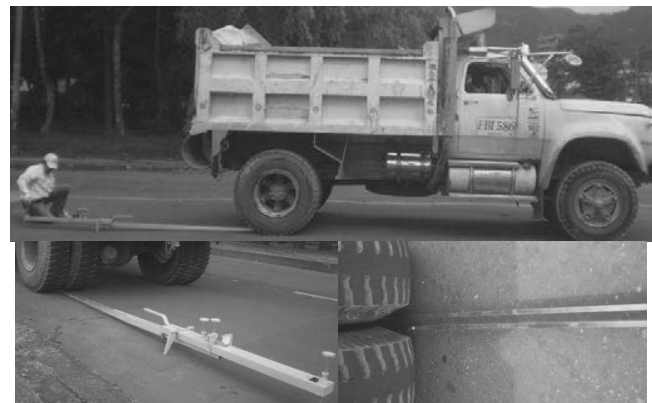
Figure 6. Benkelman beam (two-part probe beam)
