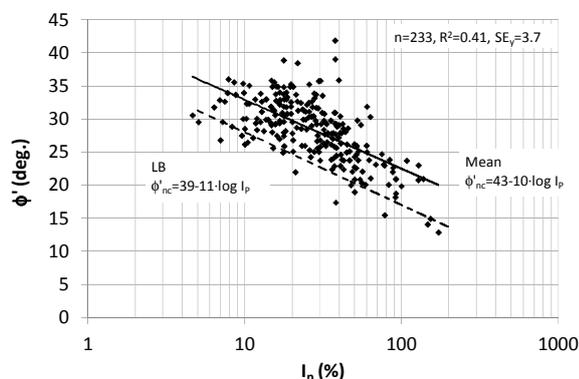
Figure 2.  $\phi'_{nc}$  vs.  $I_p$  for primarily normally consolidated reconstituted and undisturbed clays after Ladd et al. 1977 (with data from Kenney 1959 and Bjerrum and Simons 1960), Terzaghi et al. 1996 and Brooker and Ireland 1965.
