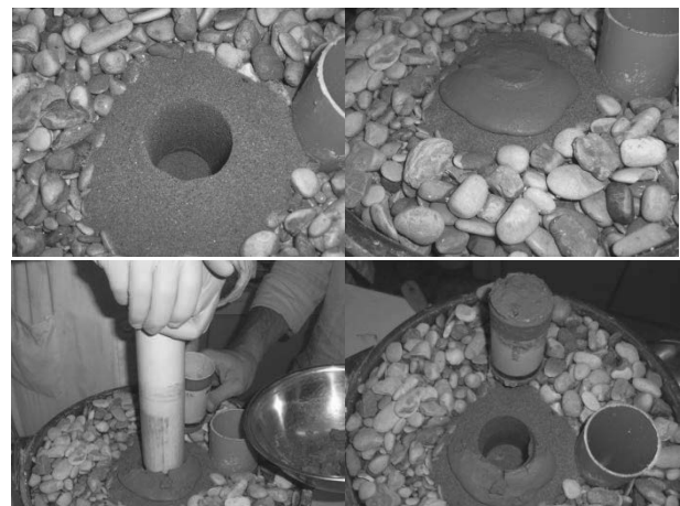
Figure 2. Experimental set-up for laboratory wet grab specimens: a) cavity preparation, b) mixture pouring, c,d) specimen retrieval.
