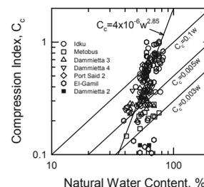
Figure.3 Data of this study on the compression index versus natural water content Terzaghi et al (1996) relationship
