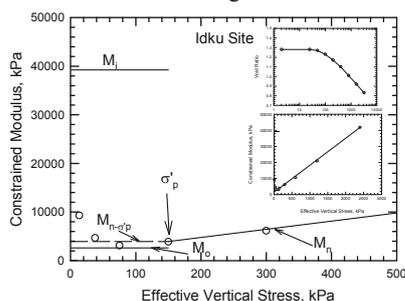
Figure 4 Definition of tangent constrained modulus concept
