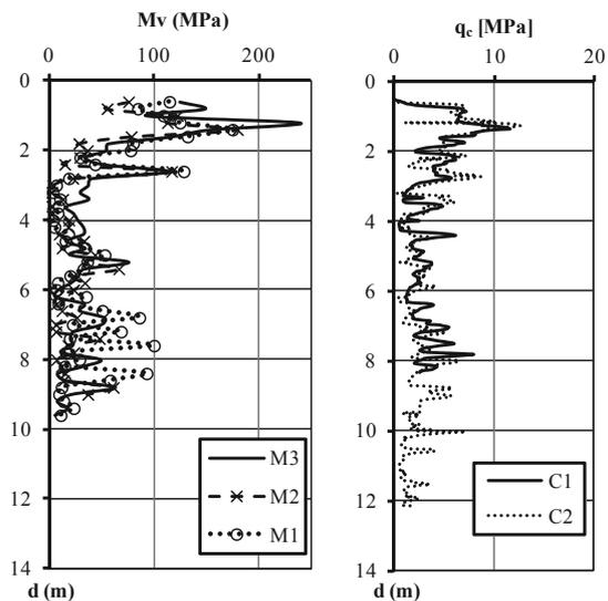
Figure 7. CPT and DMT tests in cumulative presentation
