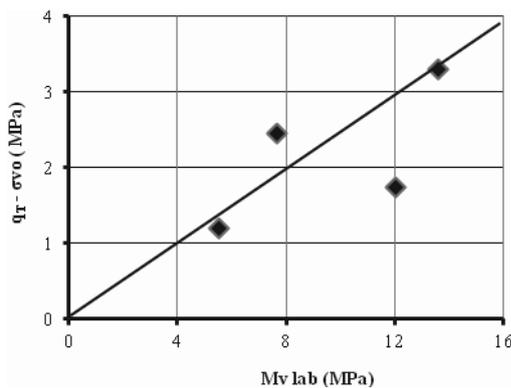
Figure 5. Relationship between laboratory determined modulus of vertical deformation and corrected tip resistance for CPT test, around B5 borehole
