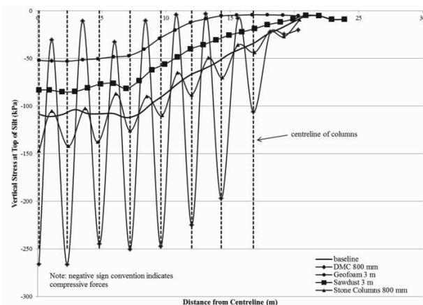
Figure 4. Comparison of predicted vertical stresses calculated at the top of the silt layer based on variable methods of ground improvements
