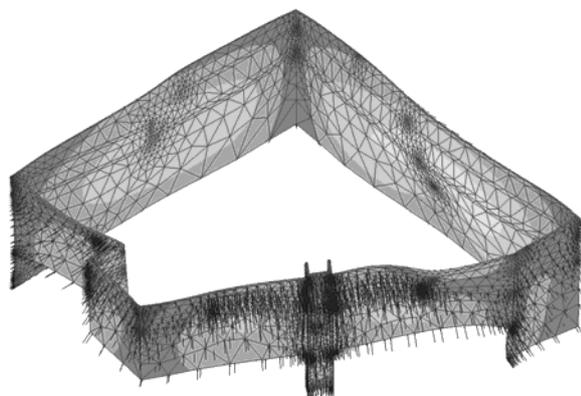
Figure 4. Deformed shape of the sheet pile wall with deflection vectors. (Deformed shape is scaled to 200 times).
