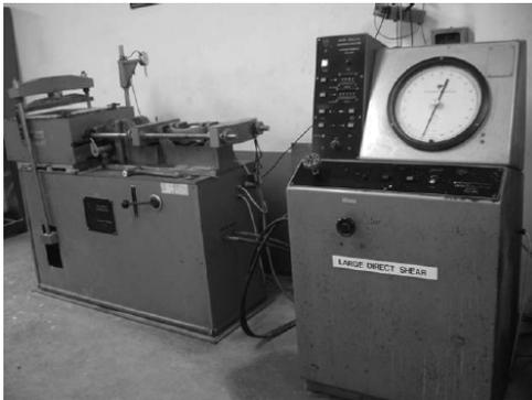
Figure 6. Large scale direct shear apparatus (Artidteang et al., 2012)
