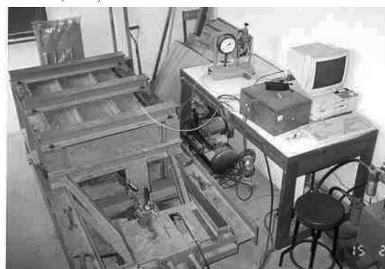
Figure 3. Pullout machine (Artidteang et al., 2012)
