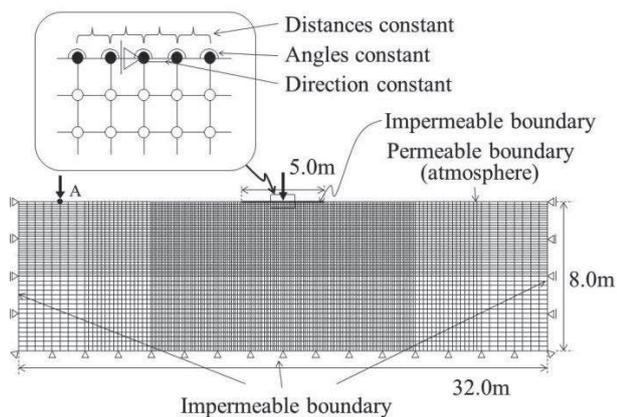
Figure 1. Finite element mesh and boundary conditions.
