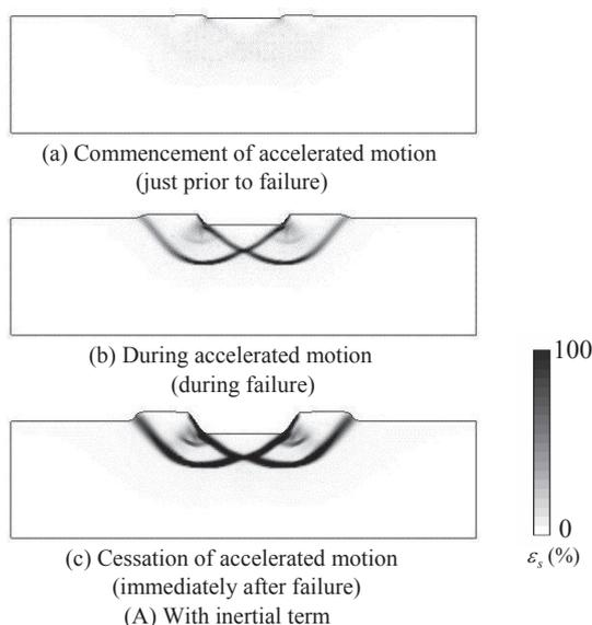
Figure 5. Shear strain distributions (load controlled case)
