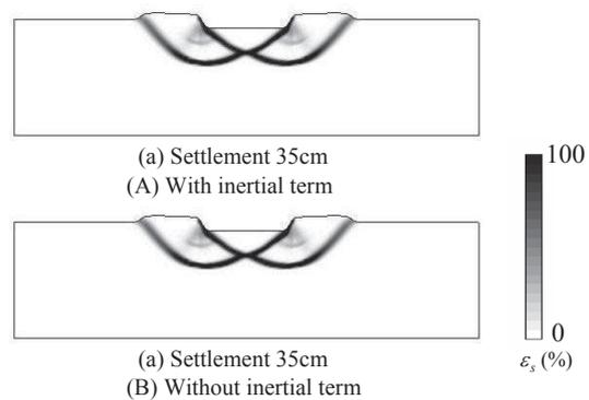
Figure 3. Shear strain distributions (displacement controlled case).
