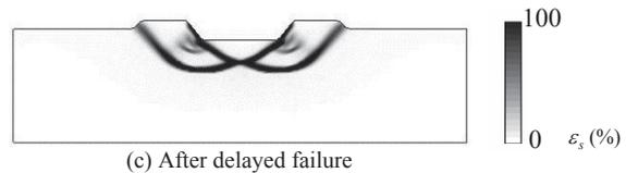
Figure 9. Distribution of shear strain (load: 128 kPa)
