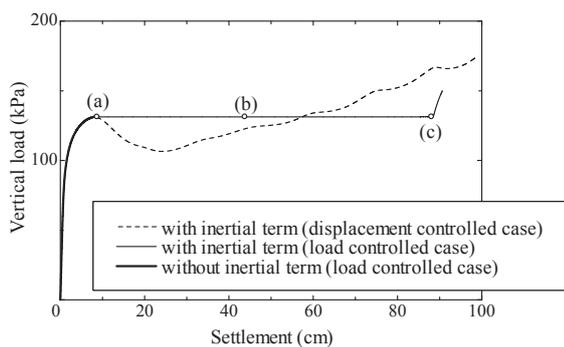
Figure 4. Relationship between vertical load and settlement (load controlled case)
