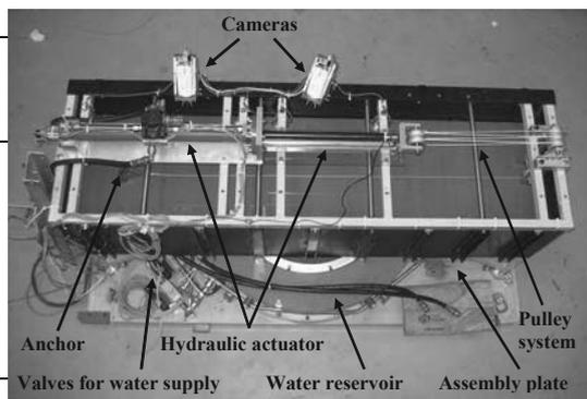
Figure 2. Anchor dragging test setup on assembly plate
