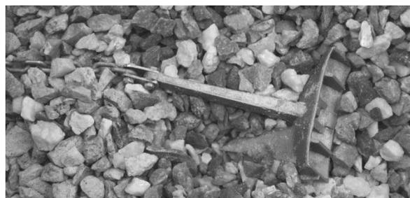
Figure 12. Position of anchor at the end of an 80-g test.
