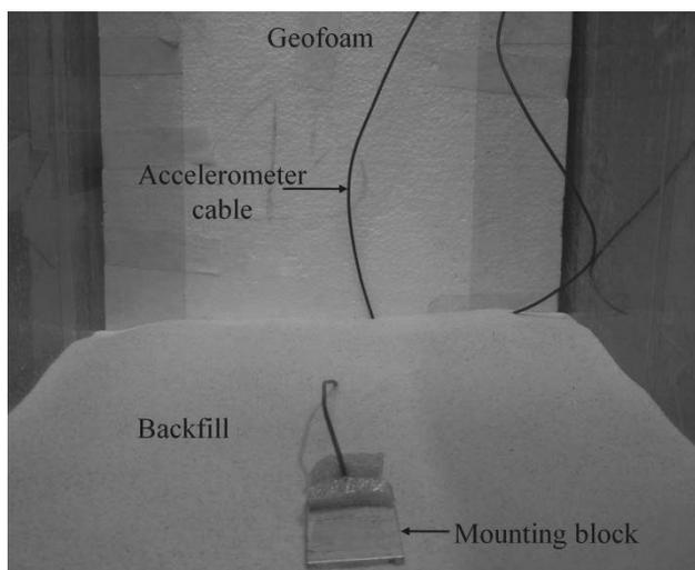
Figure 4. Positioning of Accelerometer in the backfill
