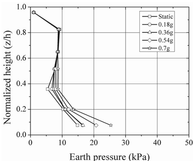
Figure 7. Earth pressure distribution for experiments with geofoam inclusion
