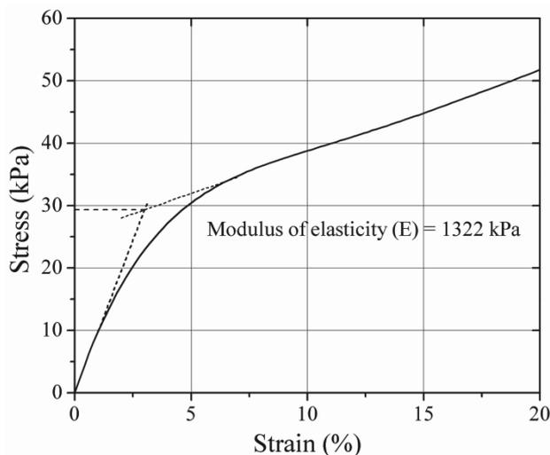
Figure 3. Stress-strain behavior of 10D EPS geofoam
