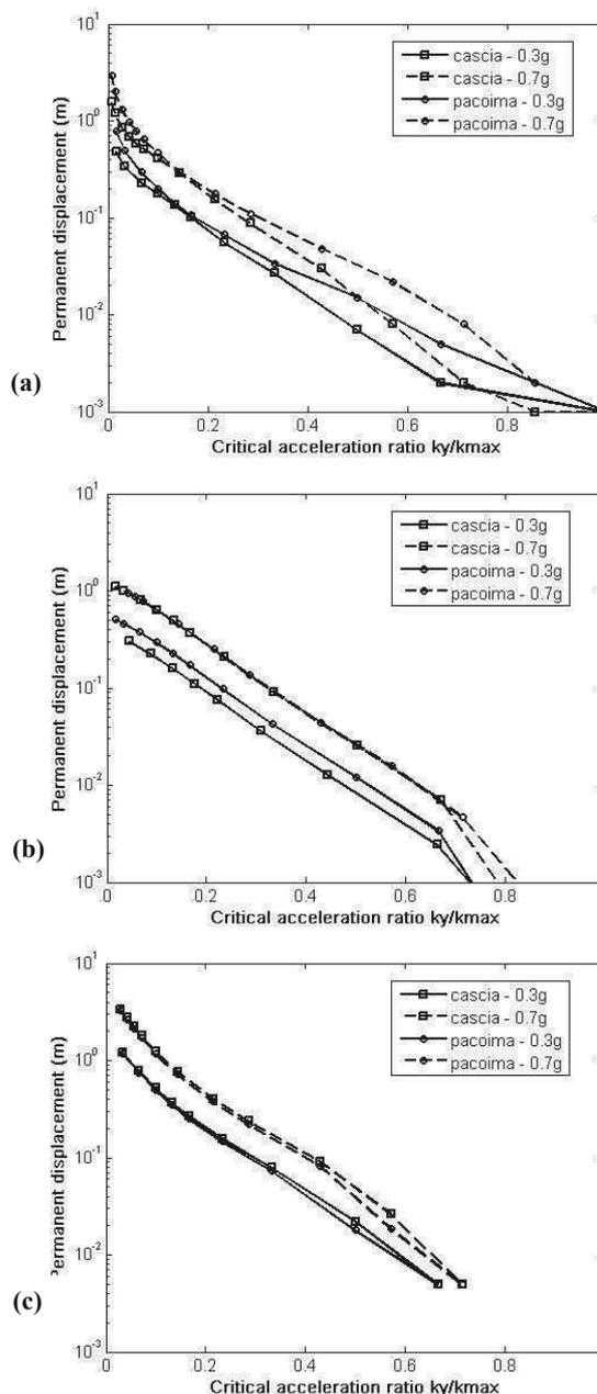
Figure 2. Newmark (a), Rathje and Antonakos (b) and Bray and Travararou (c) displacement versus  $k_y/k_{max}$  considering a nearly rigid sliding mass for different acceleration time histories (cascia, pacoima) scaled at different levels of PGA (0.3g, 0.7g)
