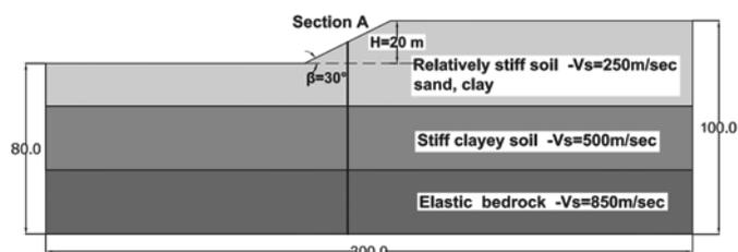
Figure 4. Slope configuration used for the numerical modeling
