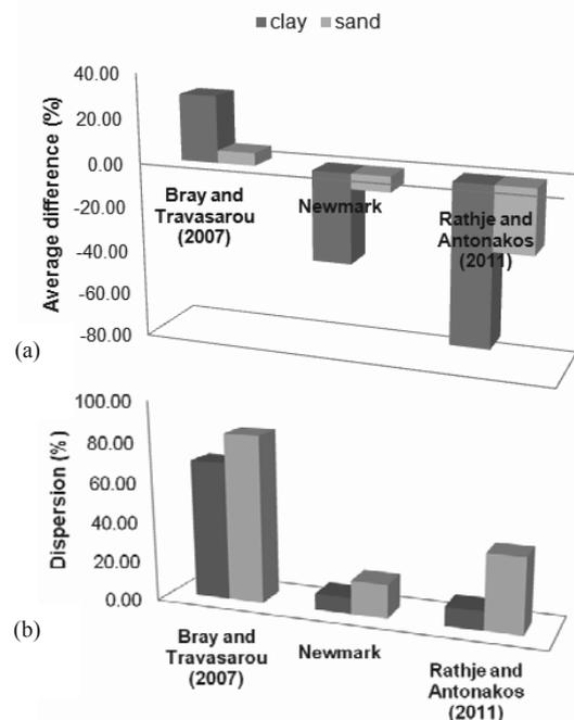
Figure 5. (a) Average difference (%) and (b) dispersion of the predictive models in the median displacement estimation compared to the corresponding numerical displacement considering nearly rigid (sand slope) and flexible (clayey slope) sliding masses
