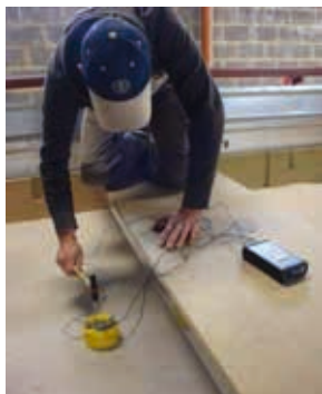
Figure 2. Impedance test using a hammer impact on the foundation.
