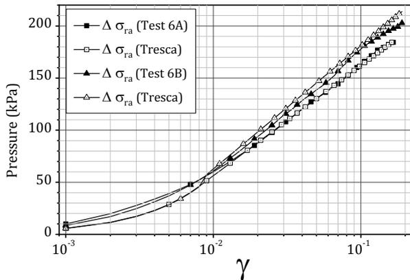
Figure 2. Comparison between experimental and Tresca-based expansion curves.
