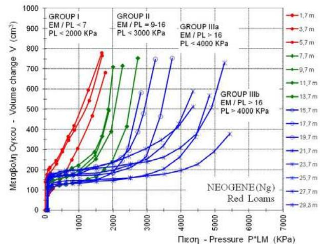
Figure 2. Red Loams (Ng) – Pressuremeter borehole 'Athmonon'.
