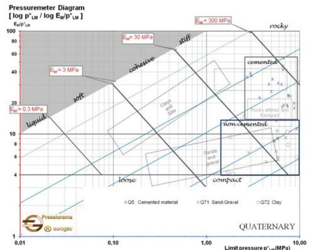
Figure 1. Pressiorama© - Quaternary, non cemented & cemented.
