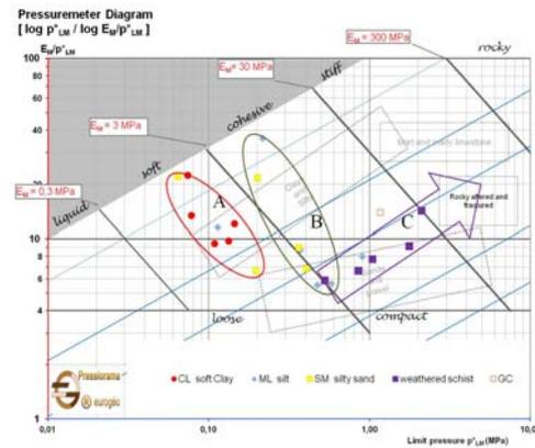
Figure 10. Pressiorama© - Offshore tests.
