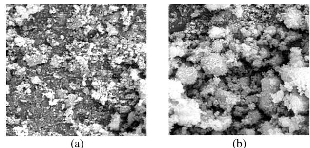
Figure 1. Images from electronic microscopy increased 5.000 times: (a) NEUT-RED-MUD 01 and (b) NON-NEUT-RED-MUD-01
