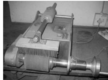
Figure 9. Abrasion test apparatus
