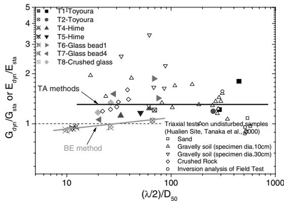
Figure 5. Effects of particle size and wave length
