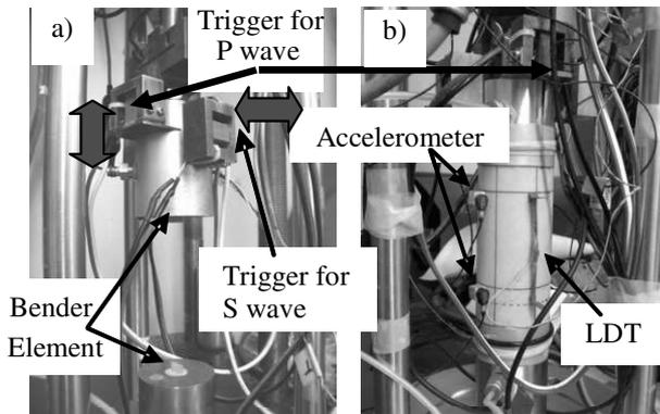
Figure 1. Specimen, LDT, Trigger Accelerometer, and Bender Element
