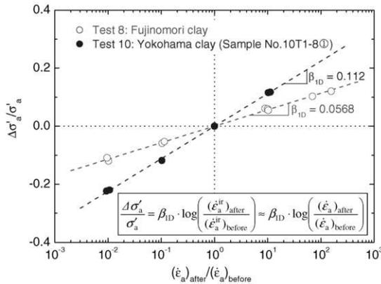
Fig. 10 Rate sensitivity coefficients,  $\beta_{1D}$
