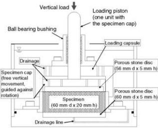
Fig. 2 Oedometer used in the present study
