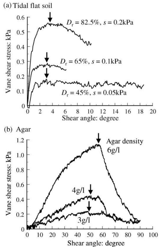
Figure 6. Results of vane shear tests on the tidal flat soils and agar.
