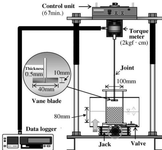
Figure 5. High-resolution vane shear system for surface materials
