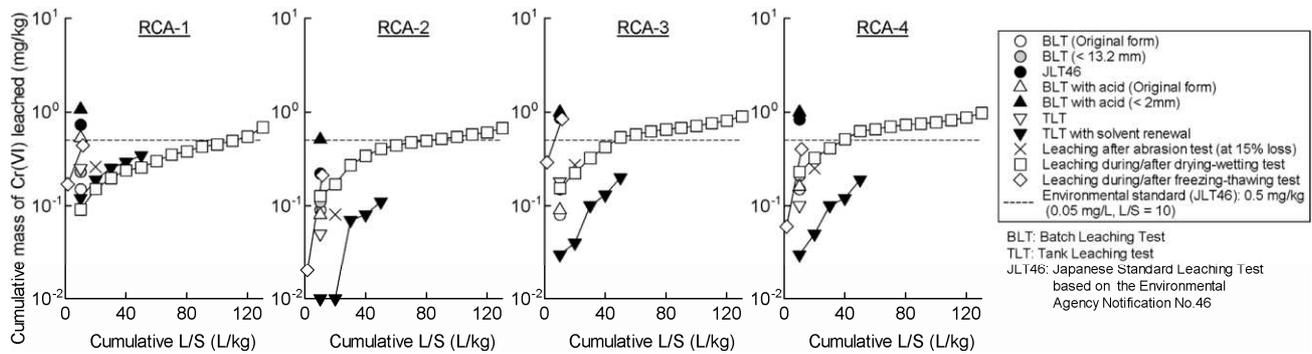
Figure 6. Comparison of Cr(VI) leaching amounts obtained in various testing methods
