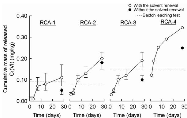
Figure 5. Mass of Cr(VI) leached in the tank leaching test.
