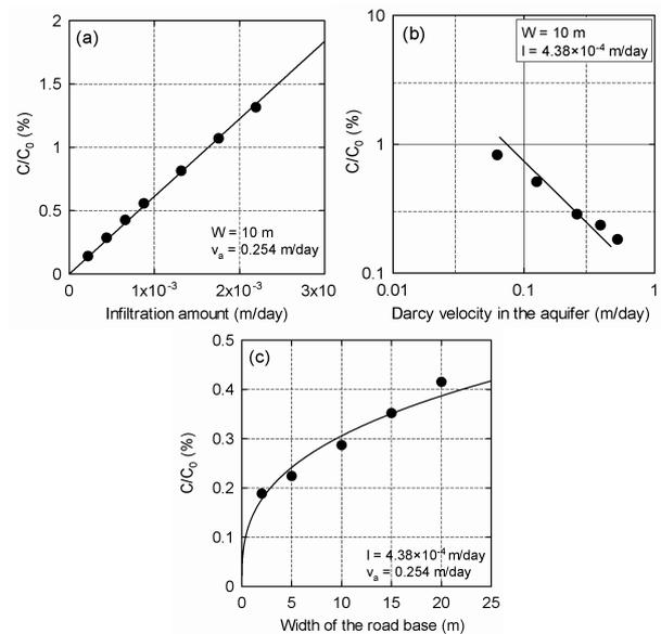
Figure 3. Effect on (a) infiltration rate, (b) flow rate in the aquifer and (c) width of the road base on the COC concentration.
