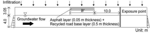
Figure 2. Cross section assumed in the analytical study
