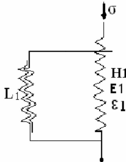
Fig.1. Rheological model representing the recoverable deformation
