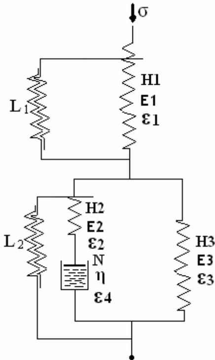
Fig.3. Complete rheological model representing a combination of springs and damping spring elements
