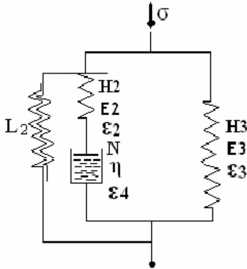
Fig.2. Rheological model representing the irrecoverable deformation
