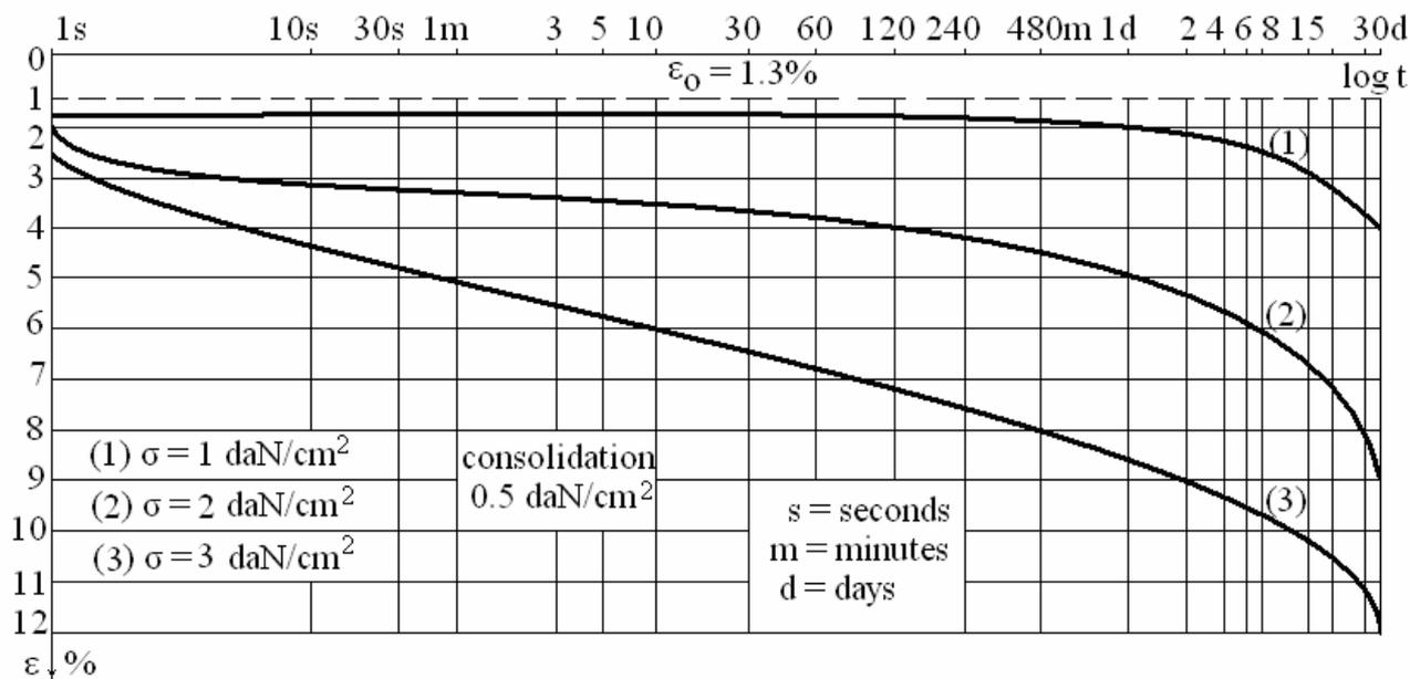
Fig.4. Creep curves on a halflogarithmic scale
